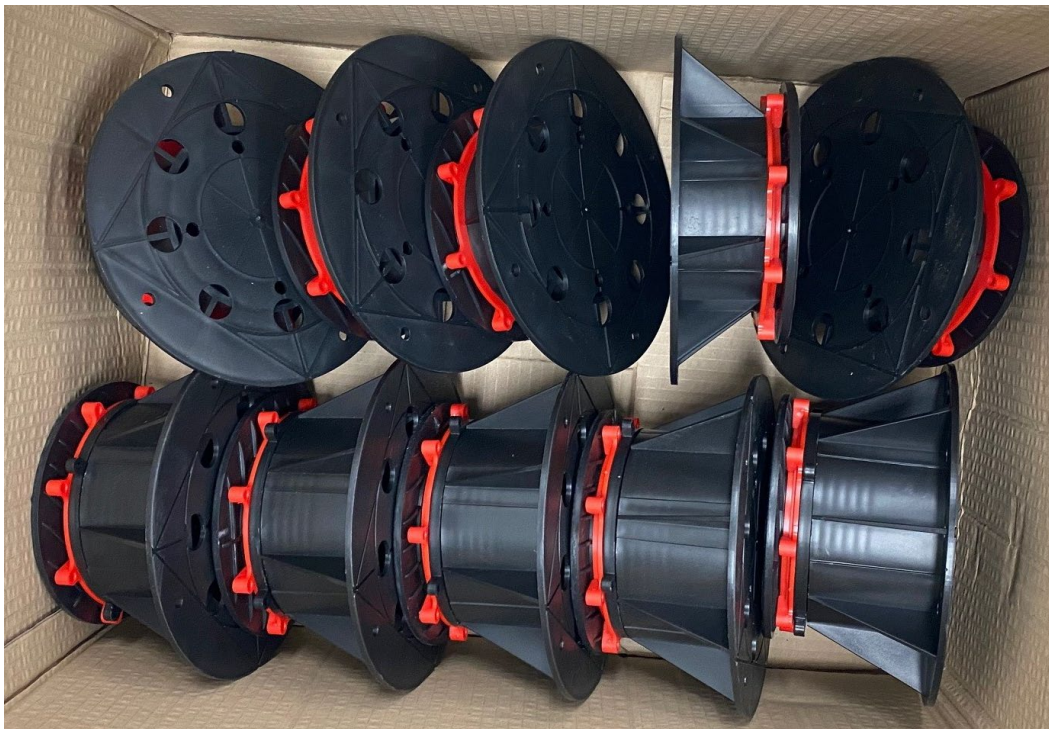
Figure 1. Pedestal samples RHN-C0-D 60-95mm (top) & Pedestal samples RHN-C0-E 95-185mm (bottom) as received by ExcelPlas
