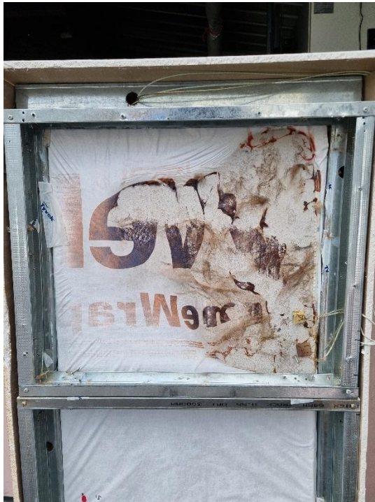
POST TEST SPECIMEN – UNEXPOSED FACE
