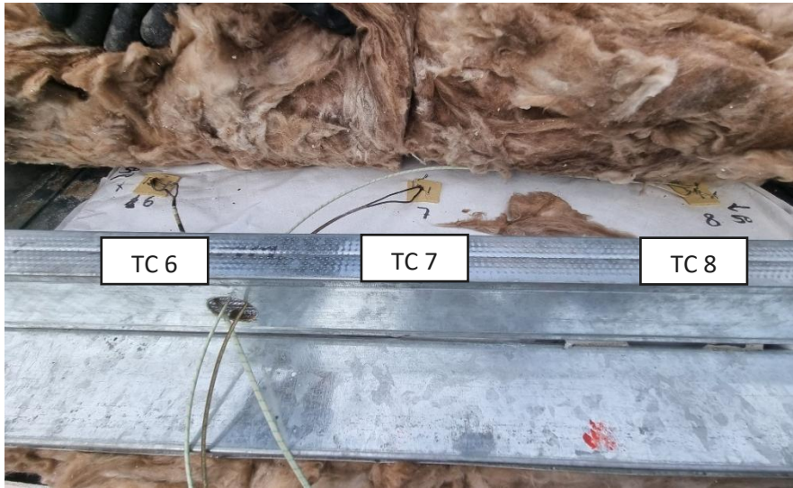
FIGURE 5: THERMOCOUPLE INSTALLATION ON THE BACK CAVITY ON SIDE CAVITY
